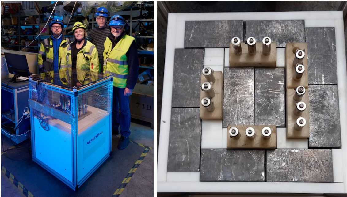
Figure 1. (Left) Photo of the fully assembled NEMESIS 1.4 setup. (Right) Configuration of the target (100 Pb bricks in 10 stacks of 10 bricks each) and fourteen helium-3 counters in PE casting. The picture was taken before adding the electronics, the external PE layer, and protective covers.
