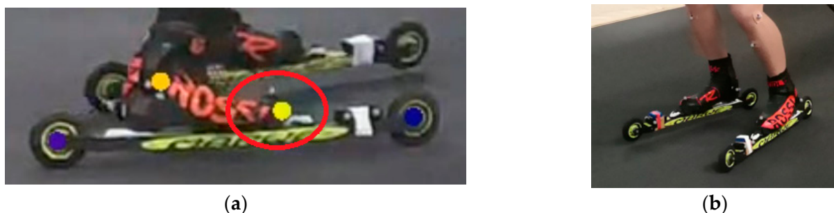
Figure 4. (a) Toe marker placements for both the markerless and marker-based systems are shown in the red circle. The markerless toe marker is indicated by the yellow circle, and the marker-based marker appears as a gray circle. (b) Marker-based toe marker placement viewed from a different direction.
