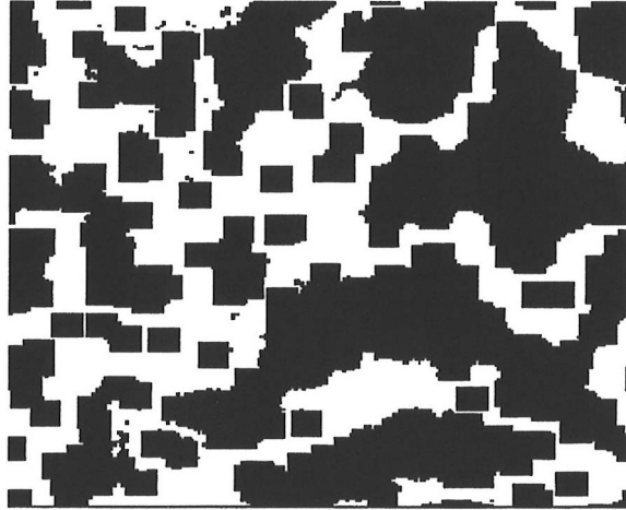
Figure 5.6: The conducting pore space of the porous sample shown in Fig. 5.5 corresponding to an effective porosity \phi_{\text{eff}} = 0.40 .
