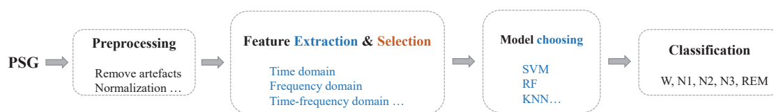
FIGURE 3 The general schematic overview of the conventional machine learning-based sleep stage classification methods.
