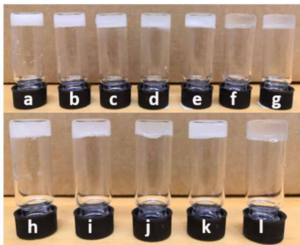
Fig. 2. Gels formed with compound 3 in: a) hexane; b) heptane; c) decane; d) tetradecane; e) cyclohexane; f) sunflower seed oil; and g) mineral oil (top). Gels formed with compound 4 in: h) hexane; i) heptane; j) decane; k) tetradecane; and l) mineral oil (bottom).
