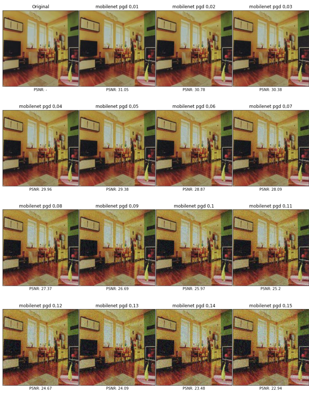
Figure 22. PGD crafted adversarial examples on image adapted from COCO dataset (Lin et al., 2017)
