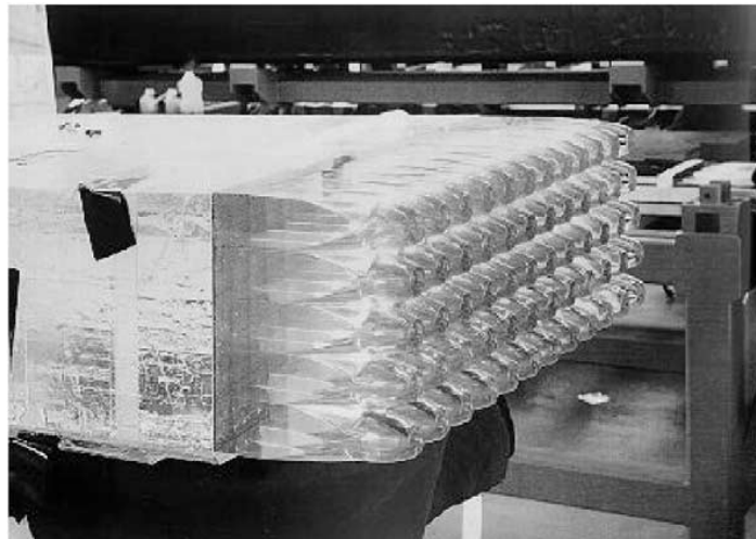
Figure 119. Light guides at one end of a barrel module before the installation of the phototubes.
