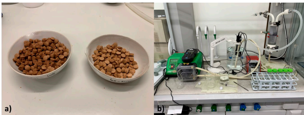
Figure 3 a) Prepared AAM blocks; b) column tests as a closed-loop system.
