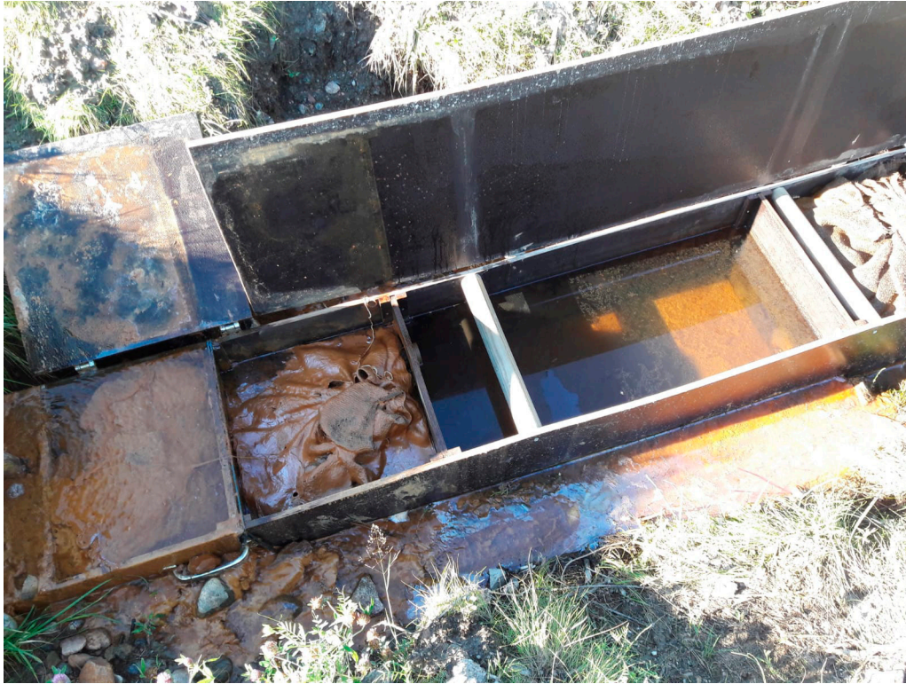
Figure 22 The field experiment of a passive barrier filtration unit.
