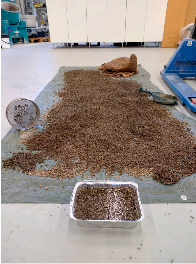
Figure 21 Semi-industrial granulation of MKGP supported on LECA.
