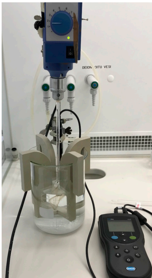
Figure 15 The equipment used in the precipitation experiments. Precipitation reactor consists of a curved blade connected to a rotor, a 2-L decanter glass equipped with stators, and a pH meter.
