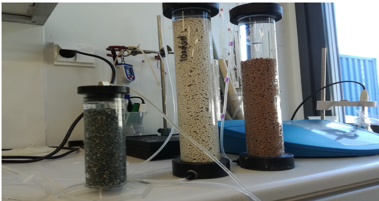
Figure 5 Adsorption columns filled with BFS-GP, FS MKGP, and MKGP adsorbents.
