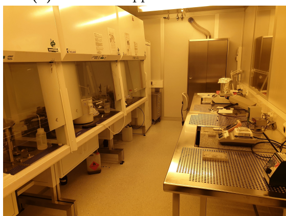
(b) Spinner cabinets and hotplates for baking resists.
