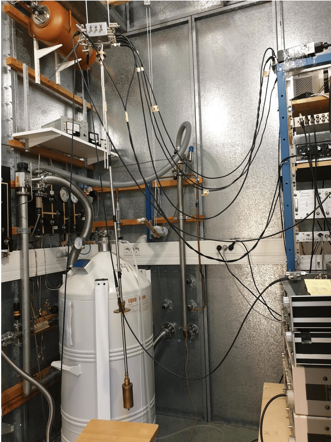
Figure 10. Dipstick measurement setup. The sample holder with the bonded chip resides in the cylinder at the bottom. The white dewar is filled with liquid helium, where the dipstick is immersed. The measurements were carried out in an electronically shielded Faraday cage.
