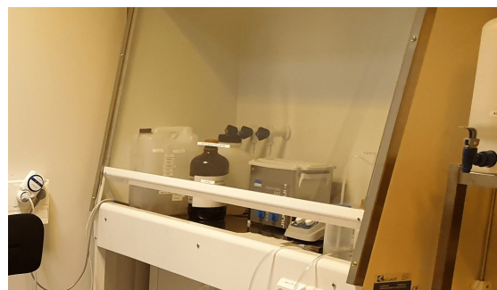
(e) Fume hood used for lift-off with sonicator.
