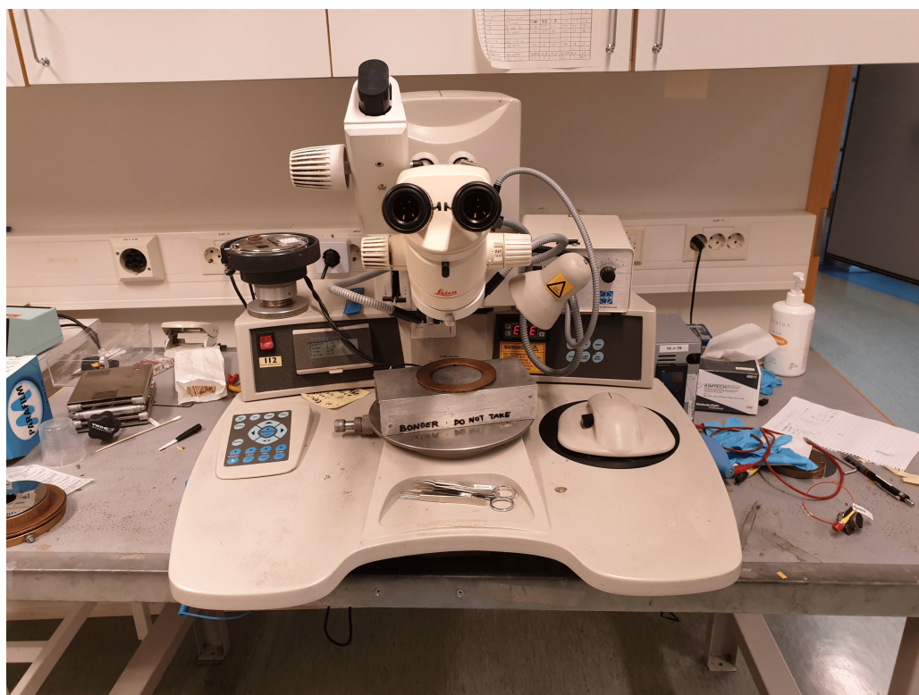
Figure 8. Wirebonder used to join the chips to the dipstick sample holder.
