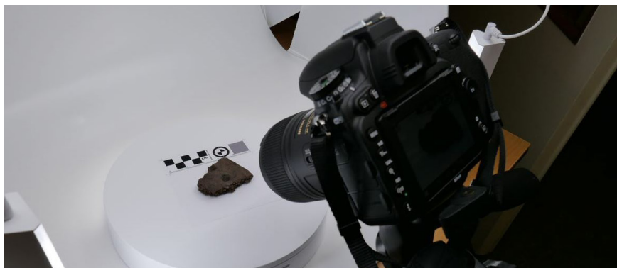
Figure 1. Creating a 3D model of a piece of prehistoric pottery with photogrammetry. The item to be digitised is placed on a rotating platform, while the camera takes digital photos of the piece from different angles. Photo: Annukka Debenjak-Ijäs.
