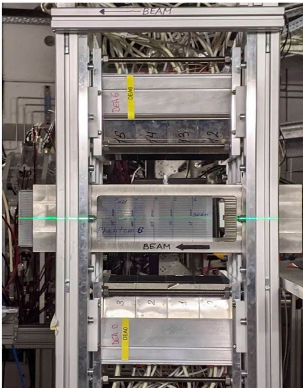
FIGURE 5 | The dual-panel UMCG positron imaging system installed at the Fragment Separator FRS at GSI. A beam of radioactive ions is coming from the right hand side and stopped in the PMMA phantom seen in the middle of the picture. The two detector panels are installed above and below the phantom each at a distance of 30 cm.
