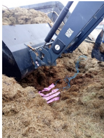
Figure 2. The farm-scale patch-reactor samples were set inside polyester bags that were set into the bottom, middle and on top of the biomasses. (Photo: Marjaana Hassani).
