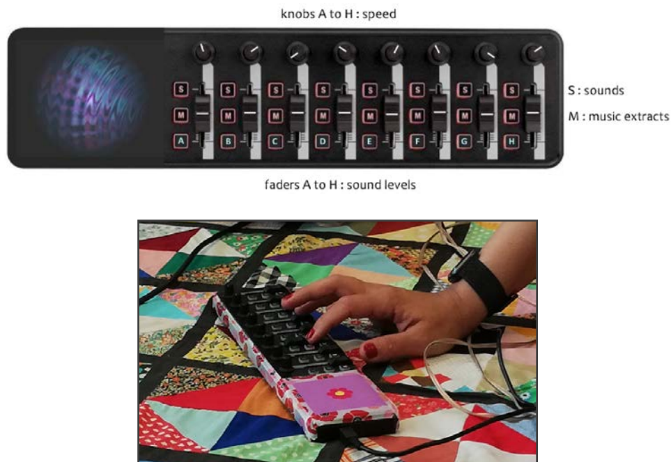
Figure 3. The MIDI interface allowed patients to manually control the stimuli, both the choice of sound and the character of that sound (i.e., sound level and speed).
