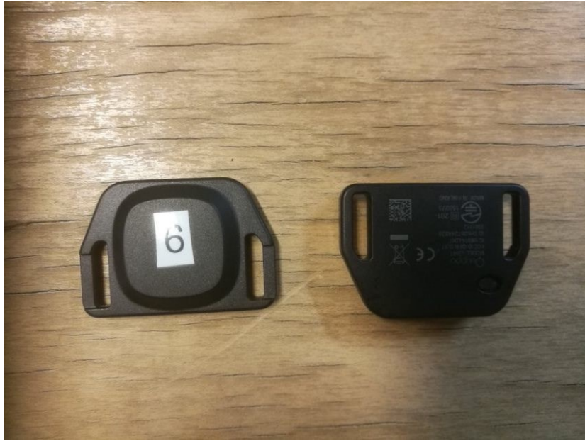
FIGURE 5. Quuppa Intelligent Locating System™ tags that were installed in the player's jerseys.
