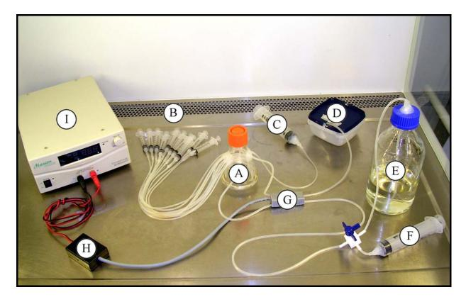
Figure 2. A: the microcosm, B: 10 sterile 5 ml syringes for sampling, C: a 50 ml storage syringe, D: Outflow tube submerged in 75 % alcohol, E: the resource stock bottle, F: a 50 ml syringe and 3-way valve for renewal of the resources, G: a heating element, H: a thermostat and I: a power supply for the heating element.
