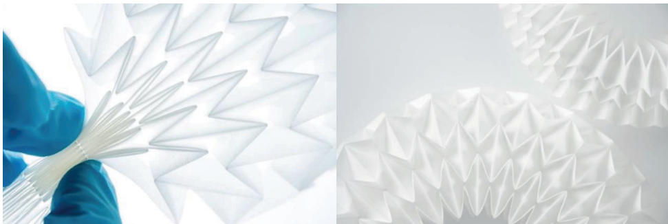
Figure P5. Different shapes of the Waterbomb tessellation pattern, designed to serve as cushioning materials. Photos by Valeria Azovskaya.
