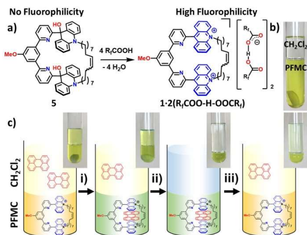
Figure 5. a) Conversion of the bis-acridane 5 to the highly fluorophilic bis-acridinium 1:2(R f COO-H-OOCR f ) ; b) Photograph of a biphasic system taken after stirring and decantation of a stock solution of 1:2(R f COO-H-OOCR f ) in PFMC ( c = 0.55 \times 10^{-3} \text{ mol L}^{-1} , 6 mL, stir bar in the bottom of the tube) and fresh \text{CH}_2\text{Cl}_2 (3 mL); c) Photographs and schematic representation of the extraction/release of Per using 1:2(R f COO-H-OOCR f ) ; i) magnetic stirring (30 min, 1000 rpm, stir bar present in the bottom of the tube) of an aliquot of the PFMC stock solution (1 mL) and a solution of Per ( c = 4 \times 10^{-3} \text{ mol L}^{-1} ) in \text{CH}_2\text{Cl}_2 (1 mL); ii) an aliquot (0.5 mL) of the PFMC solution containing Per 1:2(R f COO-H-OOCR f ) was taken and fresh \text{CH}_2\text{Cl}_2 (2 mL) was added; iii) manual shaking for 60 s and decantation.
