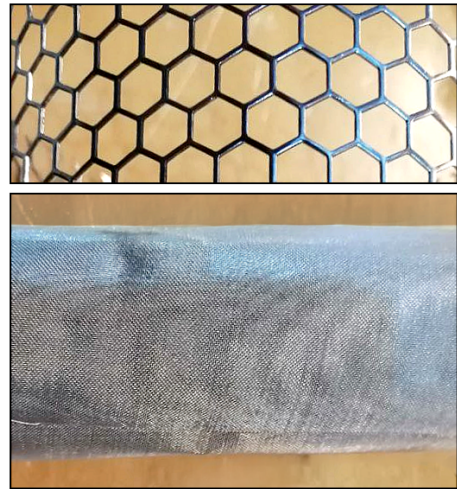
Figure 34: The two types of meshes used in this test, one very coarse and one very fine mesh. The pictures are in scale with each other.
