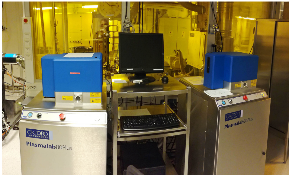
Figure 30. Picture of the Oxford Plasmalab 80+ RIE located at NSC cleanroom. The RIE vacuum chamber is seen on the left, and the one on the right is the chemical vapour deposition (CVD) chamber.
