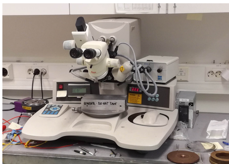
Figure 35. Kulicke & Soffa 4523A wedge wire bonder that was used to make electrical connections between the sample and the dipstick sample stage.
