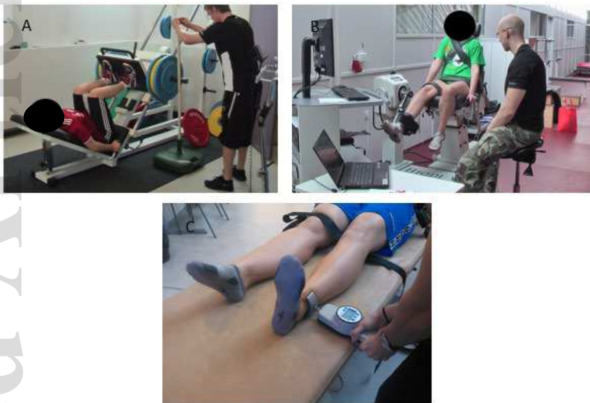
FIGURE 2 A, The measurement of maximal one-repetition seated leg press strength. B, the measurement of maximal concentric isokinetic quadriceps and hamstrings strength; C, the measurement of maximal isometric hip abductor strength
