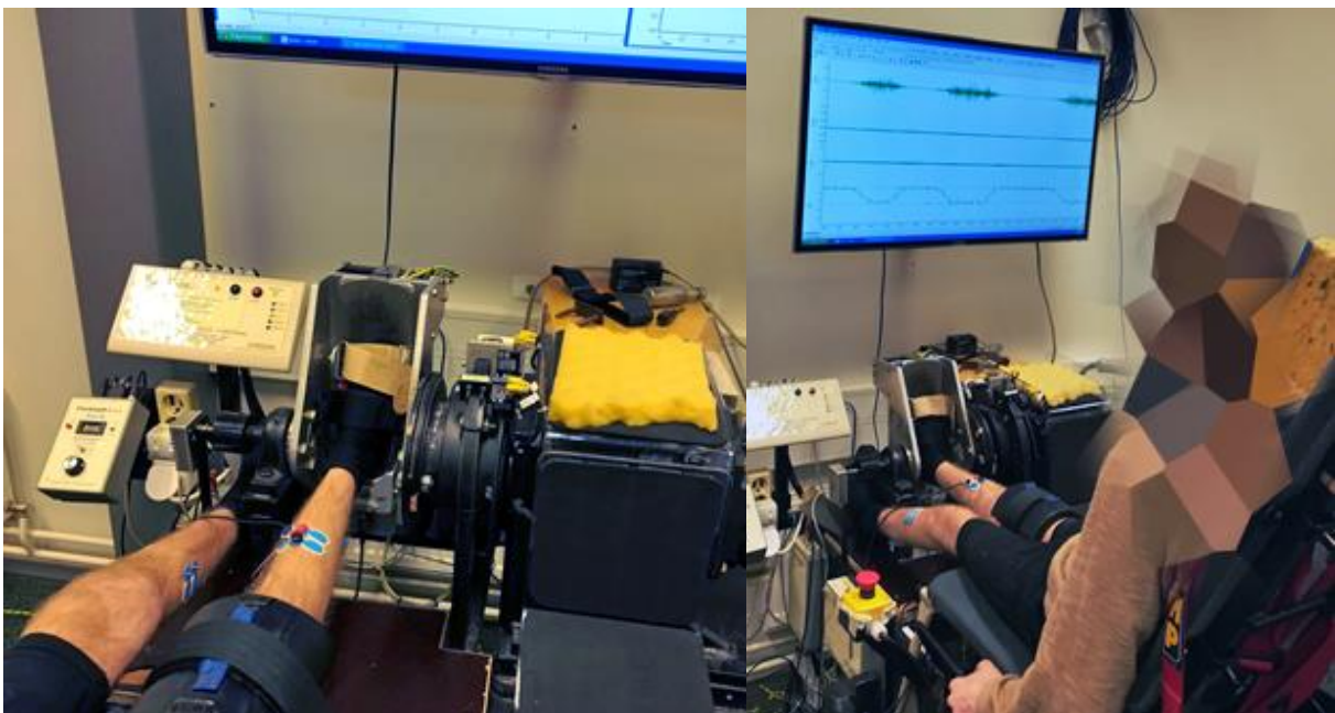
FIGURE 21. Measuring CP participant's right ankle force production in ankle dynamometer.
