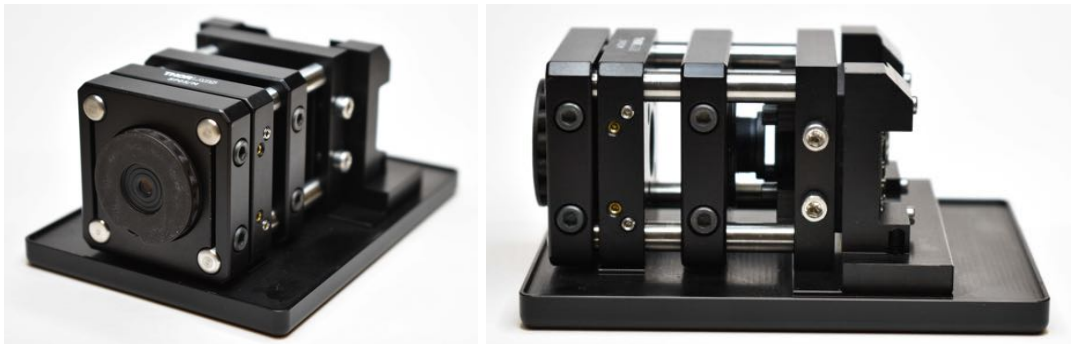
Figure 3: Interchangeable optomechanics mounted to baseplate.
