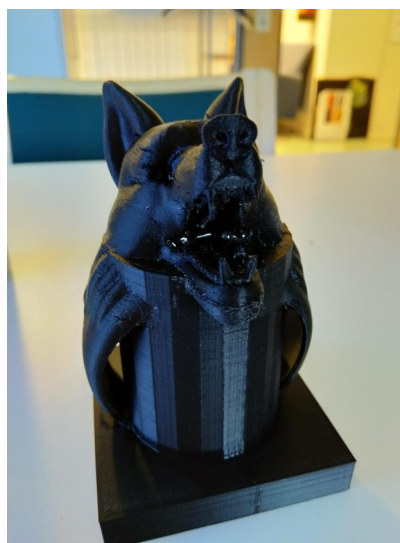
Figure 2: Ultimaker 3 Extended 3D printer producing statue (left). The statue is printed with black ABS (acrylonitrile butadiene styrene) and white water-soluble PVA (polyvinyl alcohol) is used as support material. Statue (original design grabcad.com/library/wolf-ring-1) after the support material has been dissolved (right).
