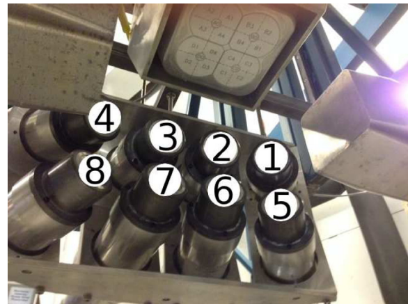
Fig. 1. (left) A schematic top-view illustration of the experimental setup. The orange arrows between the Double-Sided Silicon Strip Detector (DSSSD) and two of the LaBr 3 detectors, show that the flight paths for photons can be different as they can originate from nuclei implanted over a large area. (right) Photograph of the eight-LaBr 3 detector array together with the three clover detectors of GREAT. The identification numbers used in the text are also indicated. (For interpretation of the references to colour in this figure legend, the reader is referred to the web version of this article.)
