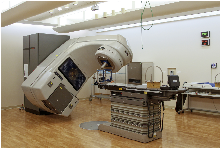
Figure 5. A linear accelerator or LINACs can be used both in radionuclide production and external radiation therapy. This figure presents a patient being prepared for external therapy with a LINAC. National Cancer Institute, Creator: Daniel Sone (Photographer) 2010; https://visualsonline.cancer.gov/details.cfm?imageid=8755 ( copied: 25.08.2018)
