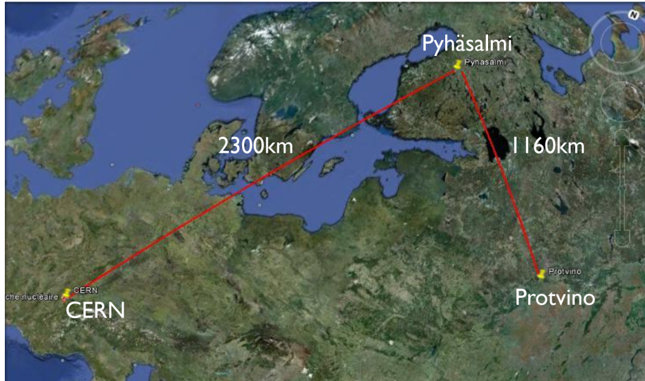
FIGURE 4.1 Schematics of the available baselines in the LBNO configuration [106]. In the plan to build LBNO, it was proposed that a neutrino beam is generated at CERN, Switzerland, whilst the detector, a large-scale liquid argon time projection chamber, would have been placed in a mine in Pyhäsalmi, Finland. An option to send a second, geometrically orthogonal neutrino beam from Protvino, Russia, was also proposed.
