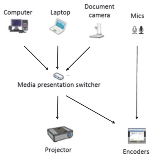
FIGURE 10 The hardware used in the recording system of the IT master's degree program
