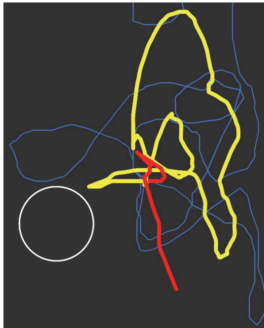
FIGURE 3 Cleanness of triggering measured as the cumulative distance travelled by the aiming point during the last 0.2 s before the shot (red line) (Mononen et al. 2003).
