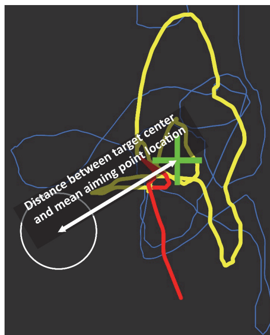
FIGURE 4 Aiming accuracy measured as the distance between target center and mean location of the aiming point (green cross) during a discrete time interval (for example 1-0 s before the shot, depicted here as yellow and red line) (Mononen et al. 2003).
