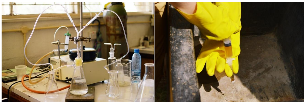
Picture 11. Solid phase extraction method was used for extraction and concentration of the water and urine samples.
