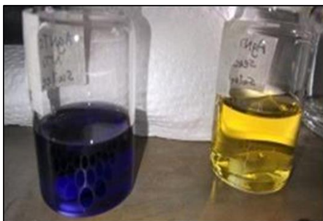
Figure 7: Aqueous colloidal dispersions of silver nanotriangles synthesized using a seed mediated process using poly sodium styrene sulfonate (PSSS).
