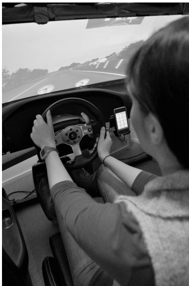
Figure 2. The driving simulation setup (without the helmet-mounted eye-tracker). The mobile device was positioned on the right-hand side of the steering wheel. Head-Up-Display (HUD) meters for speed and rpm indicated the position of the vehicle on the lane.
