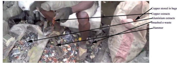
Figure 4. Smashing extraction process (also see video excerpt on Figshare.com). Source: the author.
