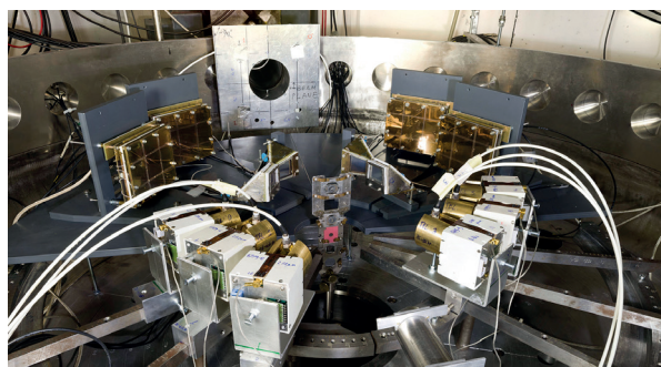
Fig. 2. Detector setup inside the Large Scattering Chamber for measuring fission-fusion reactions.
