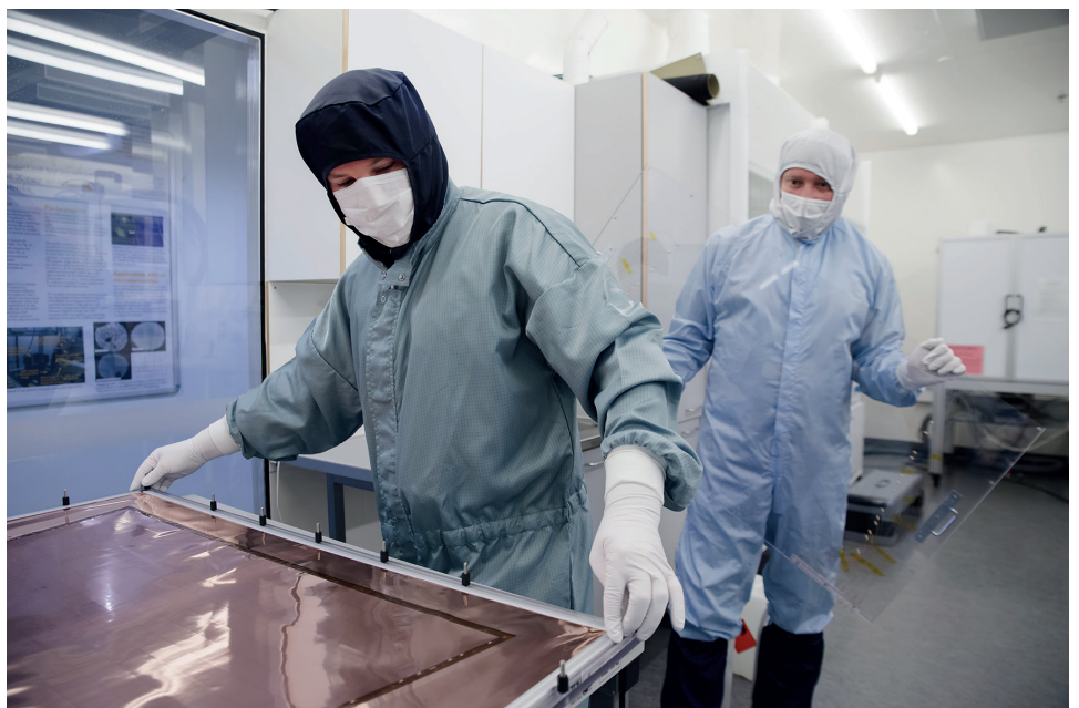
Figure 1: Members of the ALICE team inspect one of the GEM foils for the ALICE TPC ROC.
