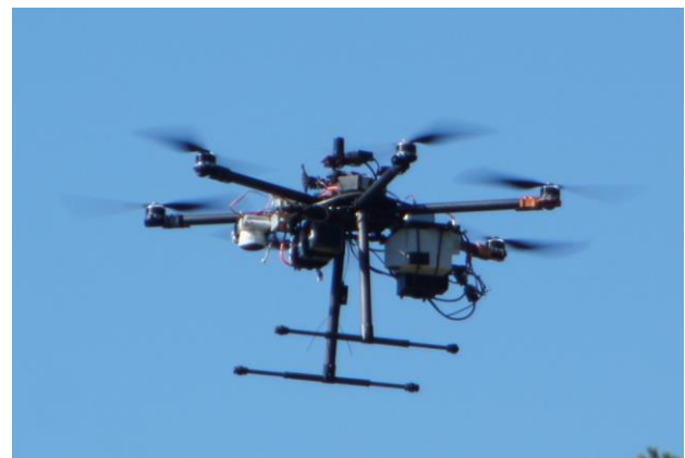
Figure 1. The UAV and the instrumentation (RGG+VNIR HS sensors) used in the UAV measurements
