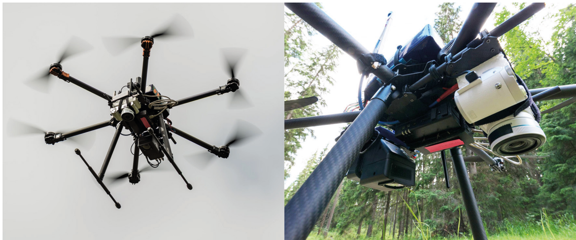
Fig. 4. UAV system (left) based on a Tarot 960 hexacopter and close-up of the sensor configuration (right) (Photographs by Tapio Huttunen).
