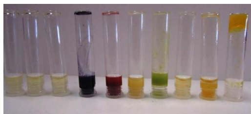
Fig. 1 From left to right 12 mM of (chloride salt of) \text{Mg}^{2+} , \text{Ca}^{2+} , \text{Mn}^{2+} , \text{Fe}^{2+} , \text{Co}^{2+} , \text{Ni}^{2+} , \text{Cu}^{2+} , \text{Zn}^{2+} , \text{Cd}^{2+} , \text{Hg}^{2+} in 6 mM of L .
