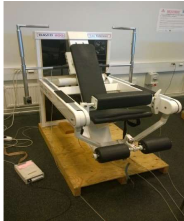
FIGURE 4. Modified David 200. Used for isometric knee extension and isometric knee flexion.
