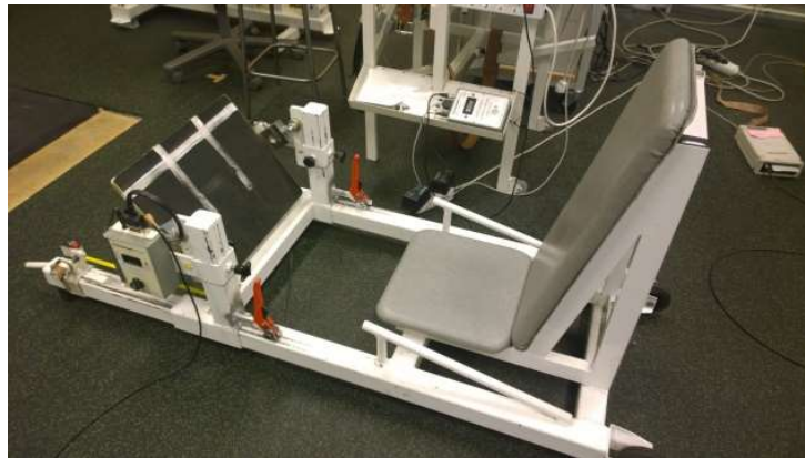
FIGURE 3. Isometric horizontal bilateral leg press, designed and manufactured by the Department of Biology of Physical Activity, University of Jyväskylä, Finland.
