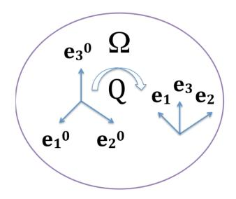
Figure 2: Transformation of global unit vectors to the local material principle vectors by rotation tensor Q.
