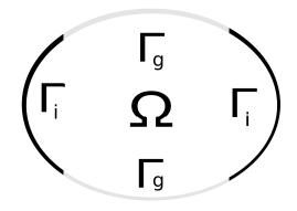
Figure 1: Domain  $\Omega$  with given temperature  $\Gamma_i$  (black) and thermally insulated  $\Gamma_g$  (grey) boundary conditions.
