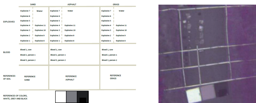
Figure 3.2: Imaging design and a hyperspectral image of airborne CBRNE detection tests
