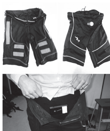
Figure 8 EMG was measured from quadriceps and hamstring muscles by textile electrodes sewed onto elastic shorts. The shorts could be worn as regular underwear with a small electronic module at the waist.
