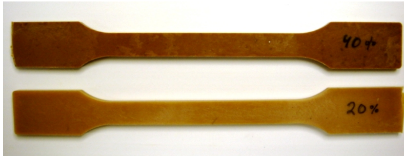
Figure 1. Tensile test specimens of birch pulp – PLA composites
