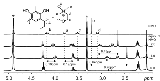
Fig. 7 Selected region of the 1 H NMR spectra (CD 3 OD, room temperature) after the addition of up to 2 equivalents of NMO to host 1 . Stars represent the residual CD 3 OD. The shift changes of the guest signals in ppm are highlighted.
