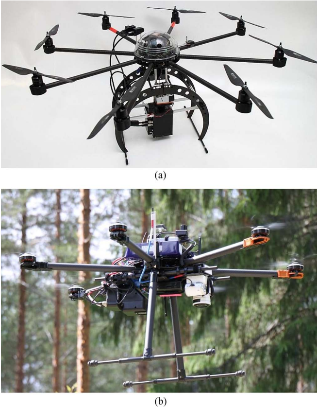
Fig. 3. (a) Lightweight SWIR camera installed in an octocopter UAV. (b) VNIR and Samsung NX300 cameras installed in a hexacopter UAV.
