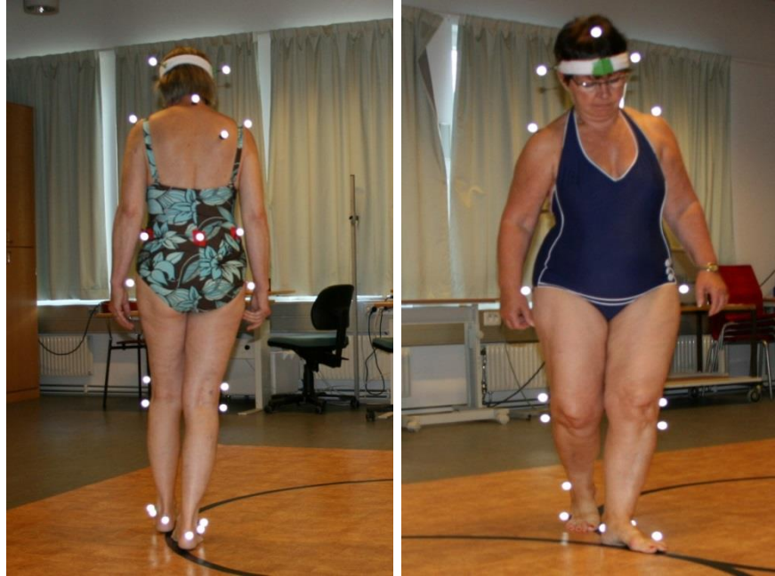
FIGURE 20. Photo of the reflective markers positioned on the PD subjects with pelvis reflector on the posterior superior iliac spine
