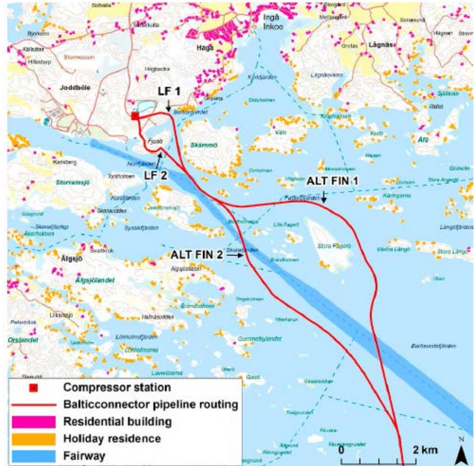
Figure O-2. The routing alternatives of the Balticconnector natural gas pipeline in Finland.
