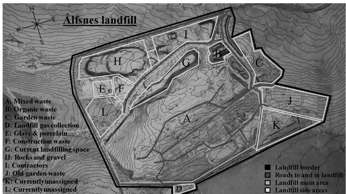
Figure 4. Álfnes landfill layout and landfilling locations of different waste fractions (SORPA 2013a).
