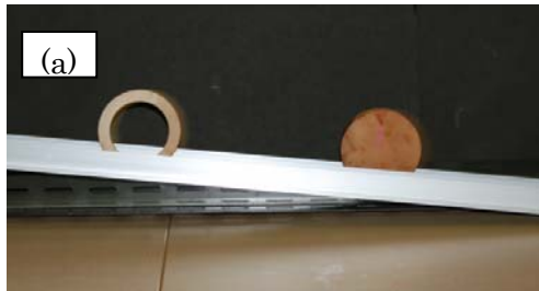
Fig.5 (a)Static figure of the demonstration in the case of Disk vs. Ring. (b)Schematic of the object rolling down a slope for explanation.
