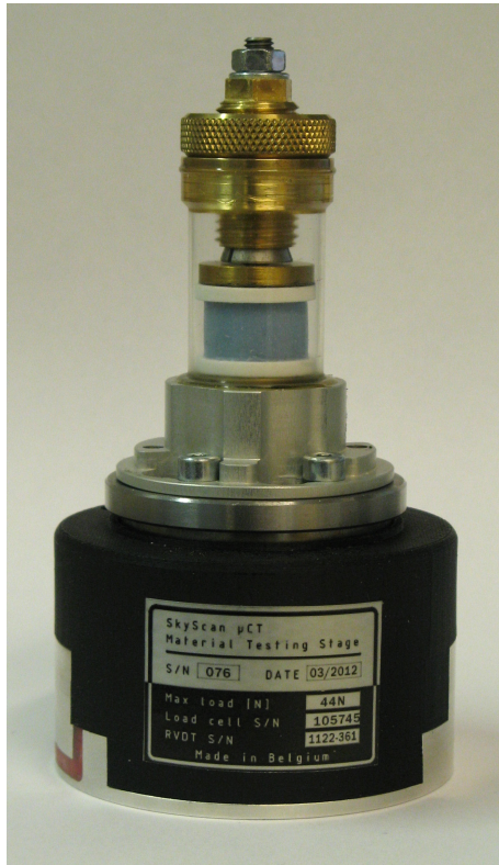
Figure 4: Sample holder (SkyScan µCT Material Testing Stage) loaded with a rubber test sample used in validating the displacement analysis algorithm.
