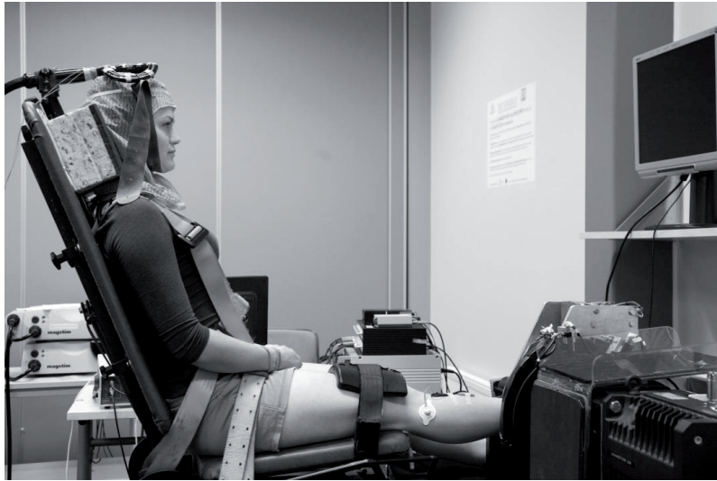
FIGURE 4 Measurement setup in the ankle dynamometer. In all experiments, participants were positioned in a custom built ankle dynamometer with the hip at 110^\circ , the knee in an extended position at 180^\circ , the ankle at 90^\circ and the right foot resting on a force pedal.
