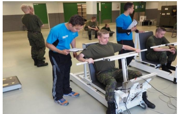
FIGURE 10. Isometric bench press manufactured by the University of Jyväskylä, Department of Biology of Physical Activity.
