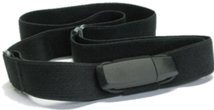
FIGURE 12. Hookie accelerometer used for measuring the loading (Traxmeet 2012.)
